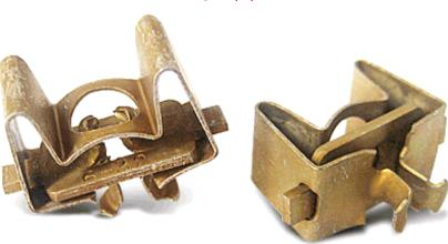
Mount aircraft instruments to the front face of the panel. Cage is easily compressed with finger-pressure to allow insertion of legs into clearance holes. When fully inserted from the back of the panel and pressure is released, legs spring apart, retaining nut in place.
