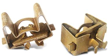
Mount aircraft instruments to the front face of the panel. Cage is easily compressed with finger-pressure to allow insertion of legs into clearance holes. When fully inserted from the back of the panel and pressure is released, legs spring apart, retaining nut in place.
